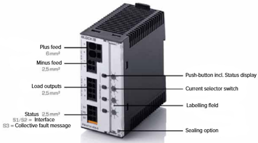
Front view with operating and display elements
